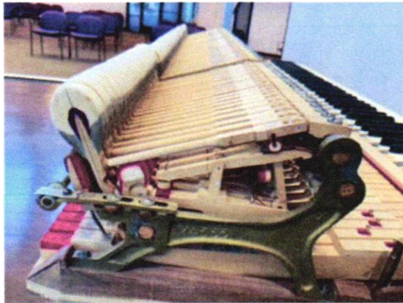
A picture of the action from both ends and overhead shots of the hammers in sections to display wear.
